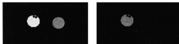
Figure 65. The spin echo images at 4.7 T and room temperature of a phantom containing \text{Dy}^{3+} - 1 and \text{Dy}^{3+} - 101 . Reference 314, Copyright 2002; Reprinted with permission of John Wiley & Sons, Inc.
